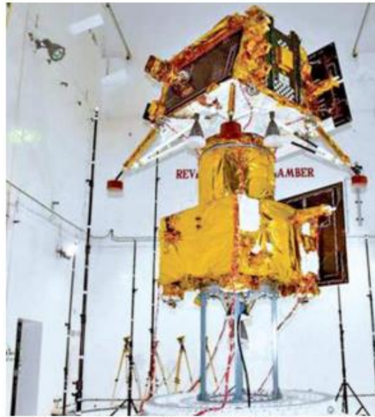
The Chandrayaan-3 propulsion module (top) attached to the lander (bottom) containing the rover, while undergoing a test, ISRO
